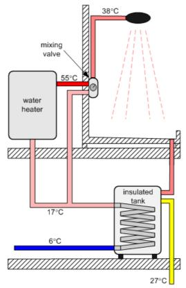
Figure 2-4: Tank based DWHR system
