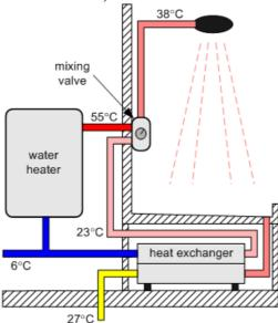
Figure 3-3: Shower mixing valve only DWHR installation
