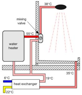
Figure 1-2: Shower setup, DWHR installed, with example temperatures
