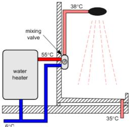
Figure 1-1: Shower setup, no DWHR installed, with example temperatures
