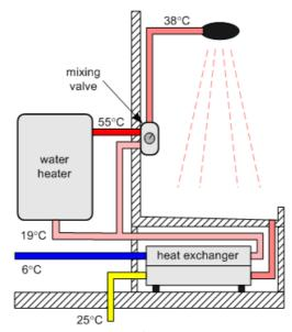
Figure 3-1: Balanced flow DWHR installation
