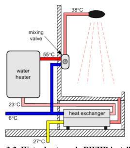
Figure 3-2: Water heater only DWHR installation
